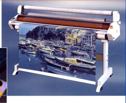
**EXCELAM COLD** is the perfect machine to procedure wide range of service in a copy shop environment or as a print Finishing. Ideal for laminating posters, ink-jet prints, leaflets and maps with superb results and for truly professional mounting up to 13mm GMP LAMIFOAM (Foamboard).
