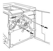
${\bf 3}$  Rotate the transfer belt release lever counterclockwise to its correct (7:00 o'clock) position.
