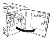
7 Insert you thumb and index finger into the two holes in the front of the toner cartridge, and then pull the cartridge straight out about 6" (15 cm).
