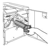
${\bf 3}$  Support the bottom of the drum with your hand, then carefully pull the cartridge toward you and remove it.
