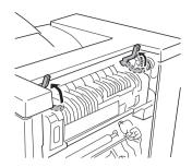
When removing the jammed media, be careful not to touch the transfer belt. Touching the transfer belt may result in poor print quality.
