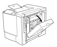
$2\,$  Remove the jammed media in the directions shown in the illustration.
