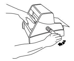
Trim to desired length using the cut blade at the roller exit. Apply downward pressure on the orange blade holder and slide to the left or right. When applying adhesive, remove the protective clear film on top to eliminate excess adhesive from around your item. Remove white liner when you're ready to adhere to your item.
