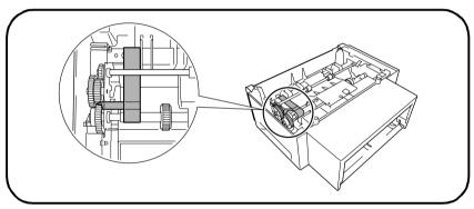
**2** Place the printer on top of the base unit. Make sure to align the coupling pins of the base unit with the holes located underneath the printer.
