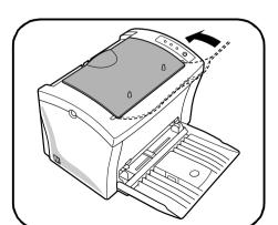
**3** Press the top cover release button and open the top cover.
