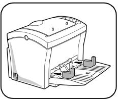
**5** Squeeze the right paper size guide and open the paper size guides. Pull out the plastic-lead strip from the paper feed inlet.
