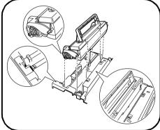
The cartridge will click into place when it is completely installed.
