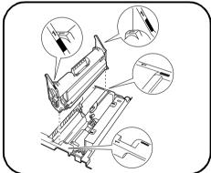
Remove the toner cartridge from the box it comes packed in. Holding it firmly with both hands, rock it in the directions indicated by the arrows in the illustration
