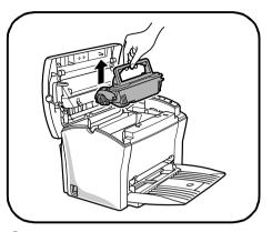
6 Install the drum cartridge into the printer, aligning the guides of the cartridge with the grooves inside the printer.
