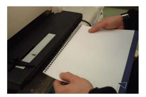
13.5 To complete the insertion, twist both ends by 90° so that the open part of the WIRE-O® faces you. The book is then ready for transfer to the closing section.
