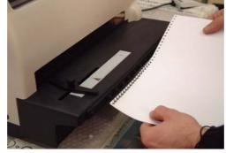
13.4 Whilst holding the first few loops, stroke the remaining loops of WIRE-O® with the other hand so that they drop easily into all the holes of the sheets.
