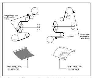
Do not allow the adhesive side of the film to contact the Heat shoes, Nip Rollers or Pull Rollers. Liquefied or tacky
