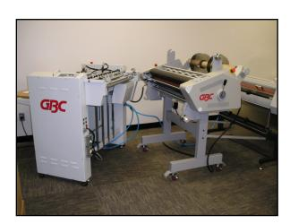
Swing out feeder to load bottom film roll.
