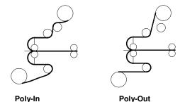
The top and bottom rolls of laminating film must be of the same width and be present simultaneously. A small amount of adhesive will "squeeze out" during lamination, where the top and bottom rollers meet at both sides of the film web. Hardened adhesive deposits can damage the nip rollers. To avoid any damage, preheat the rollers before cleaning them.
